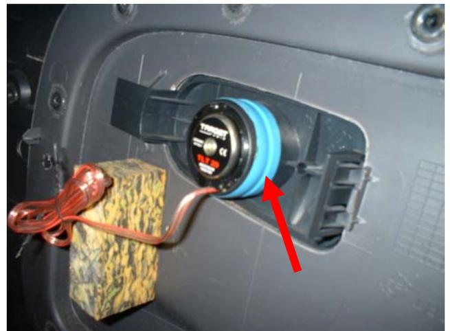
SMONTARE IL SUPPORTO DEL TWEETER E INCOLLARE IL TWEETER CON IL MASTICE AL SUPPORTO.
